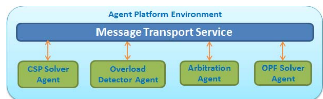
Fig. 1 Schematic diagram of MAS for ANM
